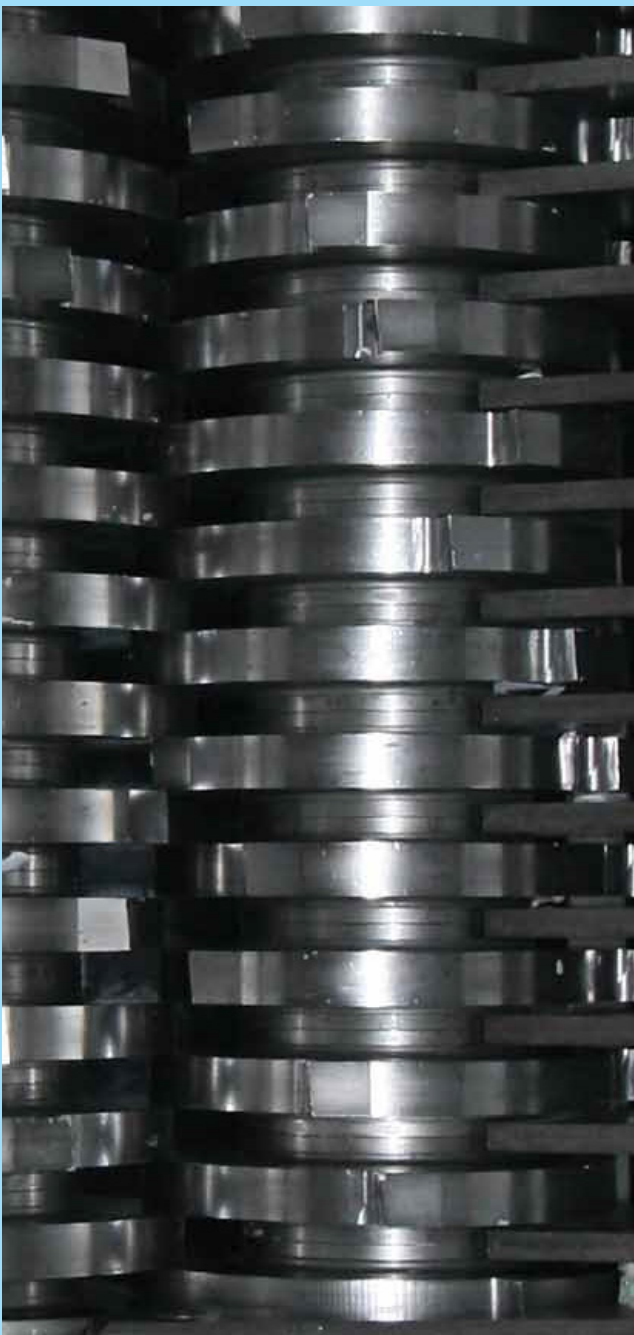
ST-10E uses 42 durable hardened steel cutting knives
